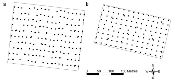
**Figure 1.** Sampling strategy used in (a) Coonawarra and (b) Sunraysia. Note that a regular grid forms the basis of (a), but with sampling points randomly removed from 30 of the grid nodes and re-allocated to vines adjacent to other grid nodes; the latter were also randomly selected. See text for further explanation.
